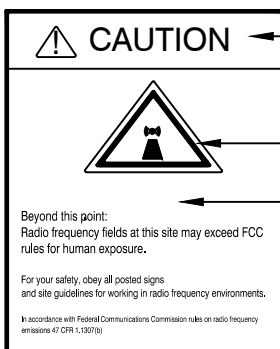
5 CAUTION-RF SIGN (YELLOW) 12" WIDE X 18" HIGH
