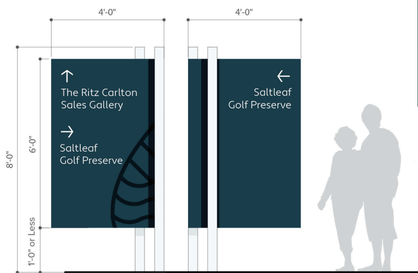
ON-SITE DIRECTIONAL SIGNS Scale : 3/8"=1'
