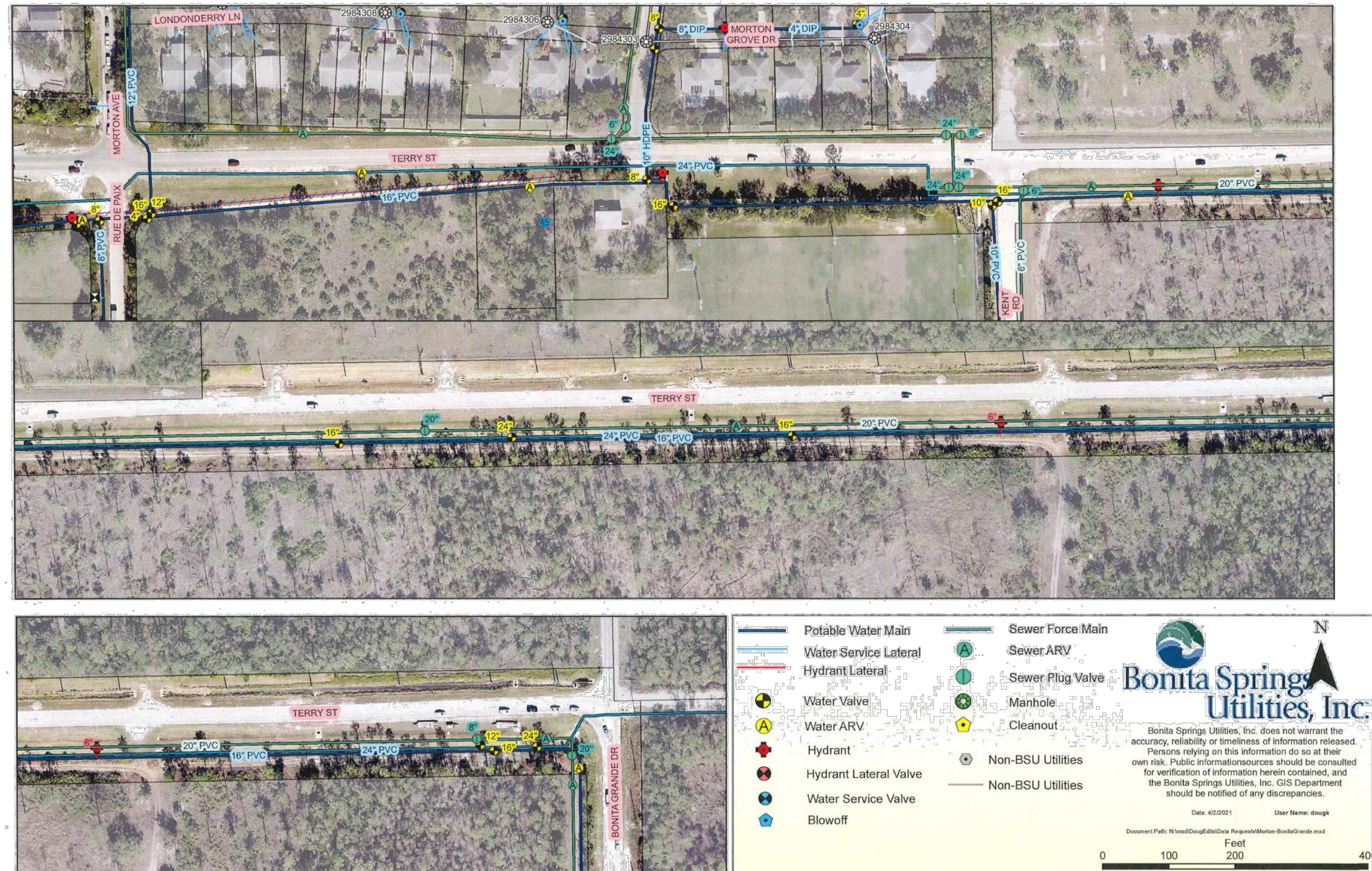
Figure 9 : Existing Utilities Plan
