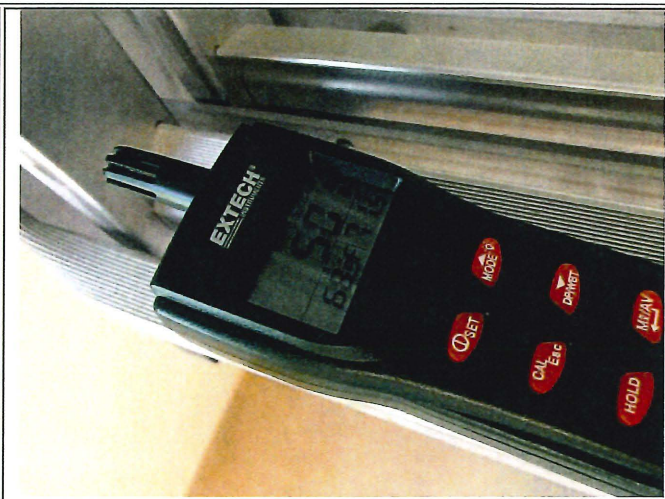
Photo 10: Break Room – Overview of temperature, relative humidity and carbon dioxide readings.
