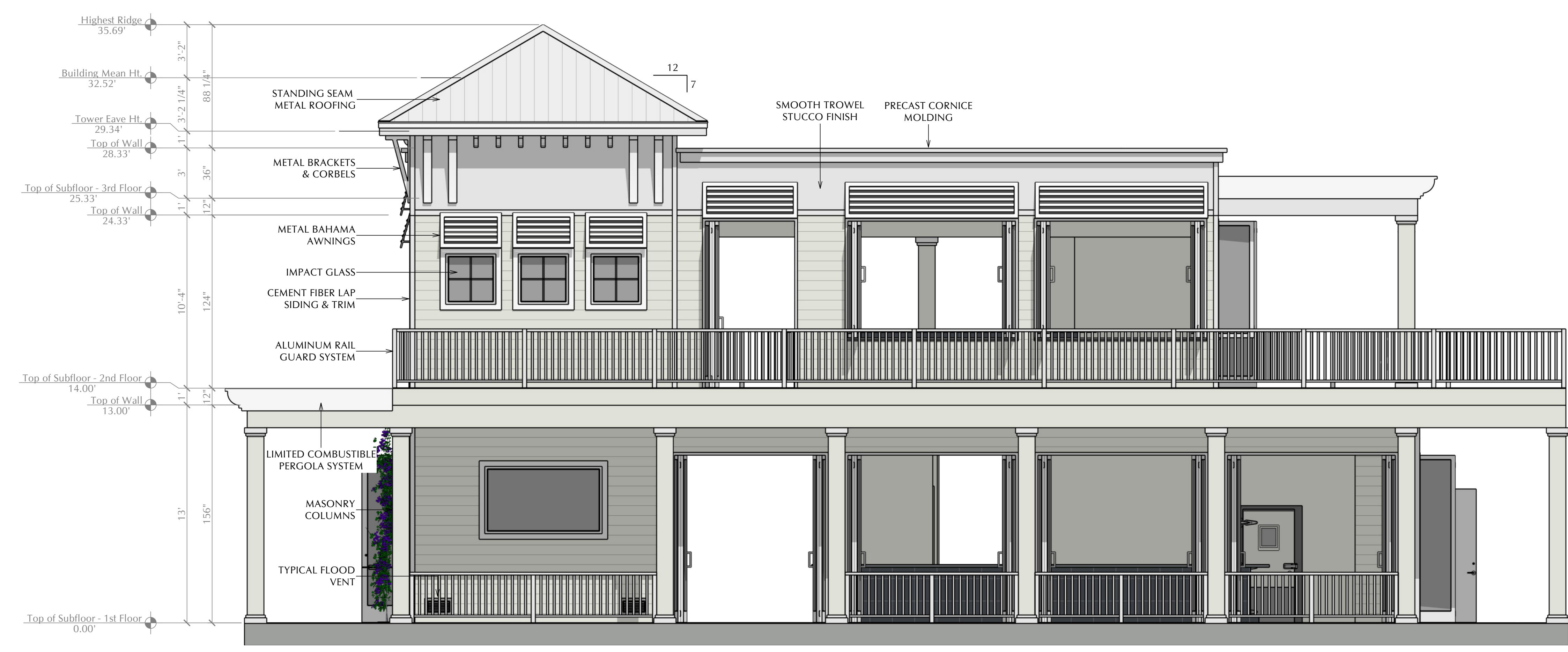
E1 - FRONT (WEST) ELEVATION Scale: 1/4" = 1'-0"
