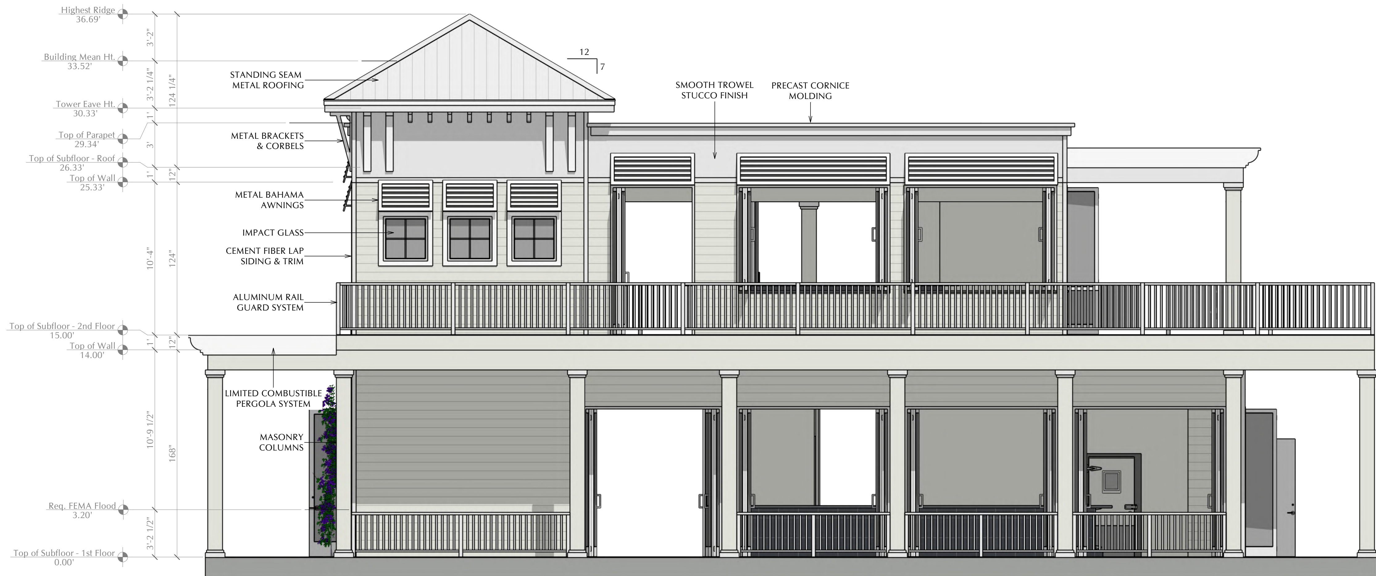
E1 - FRONT (WEST) ELEVATION Scale: 1/4" = 1'-0"
