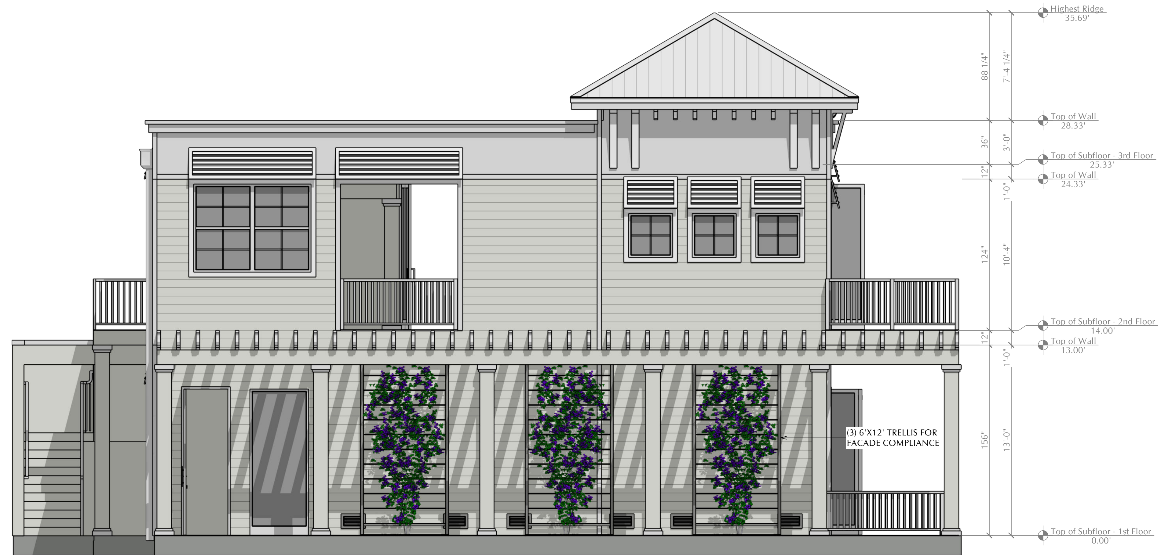
E2 - LEFT (NORTH) ELEVATION Scale: 1/4" = 1'-0"
