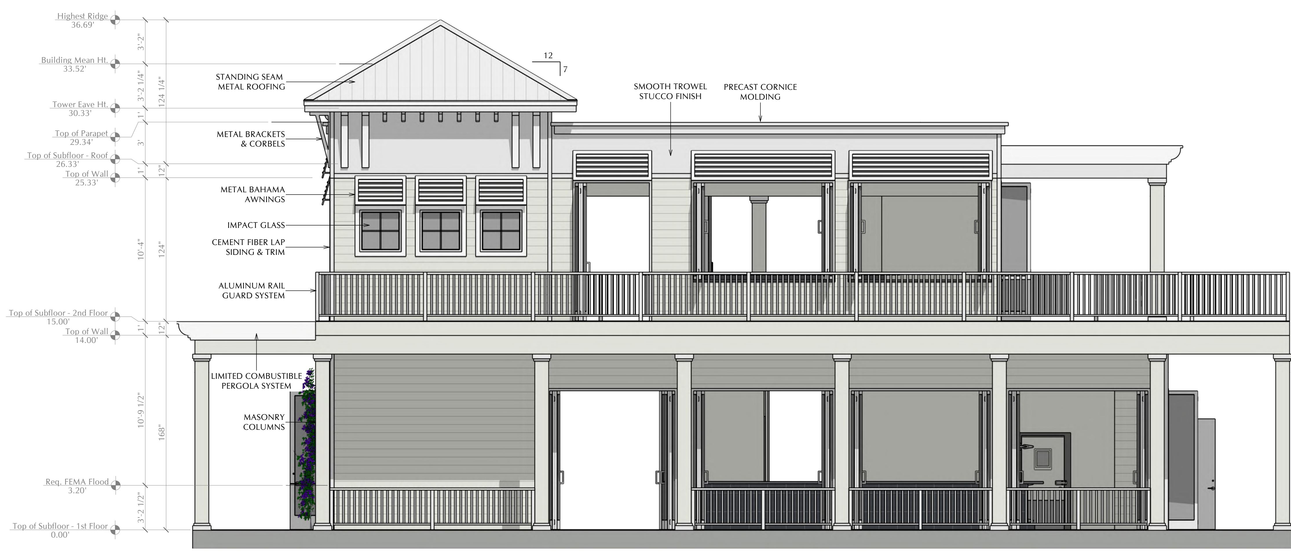
E1 - FRONT (WEST) ELEVATION Scale: 1/4" = 1'-0"
