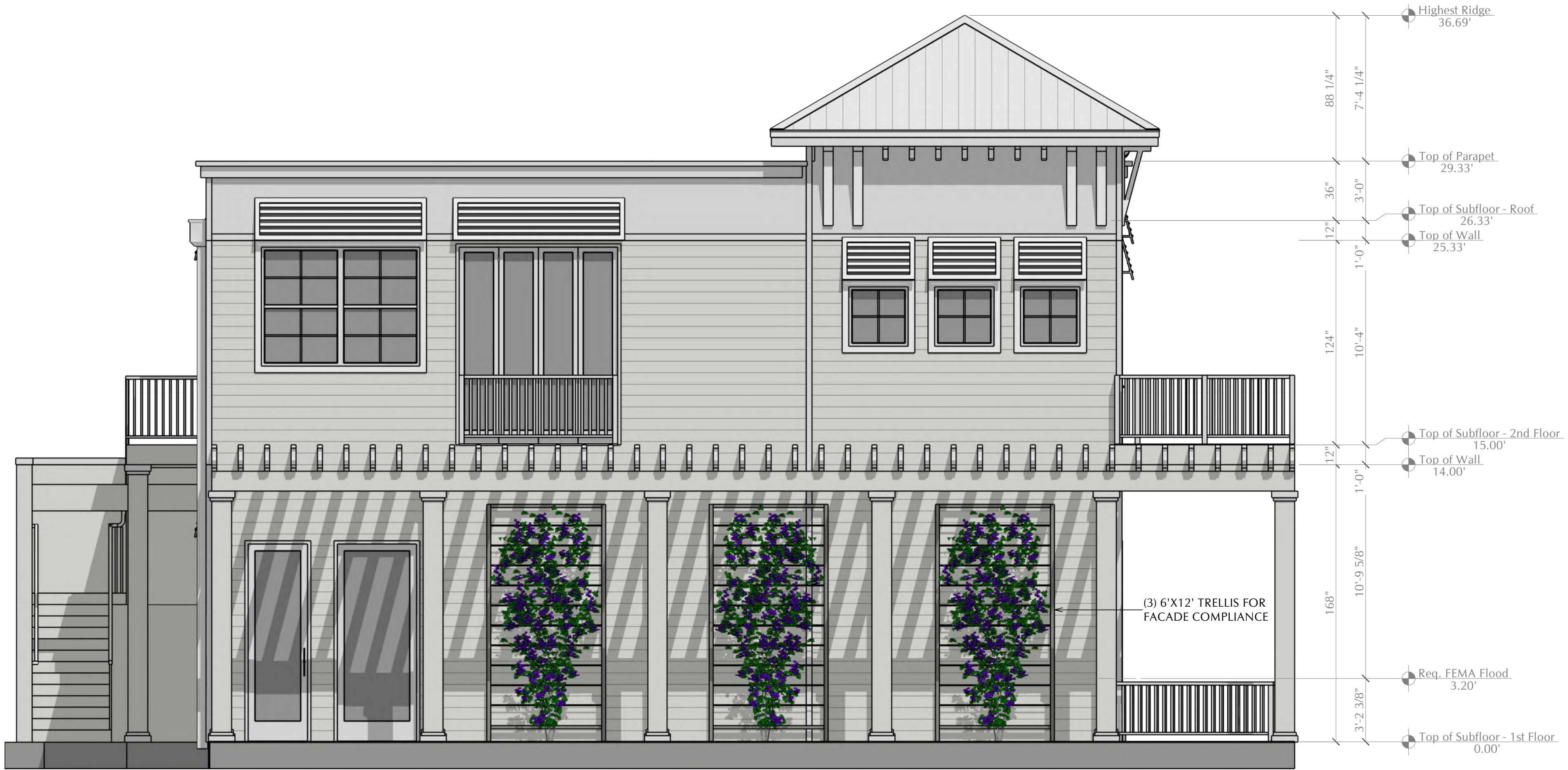
E2 - LEFT (NORTH) ELEVATION Scale: 1/4" = 1'-0"
