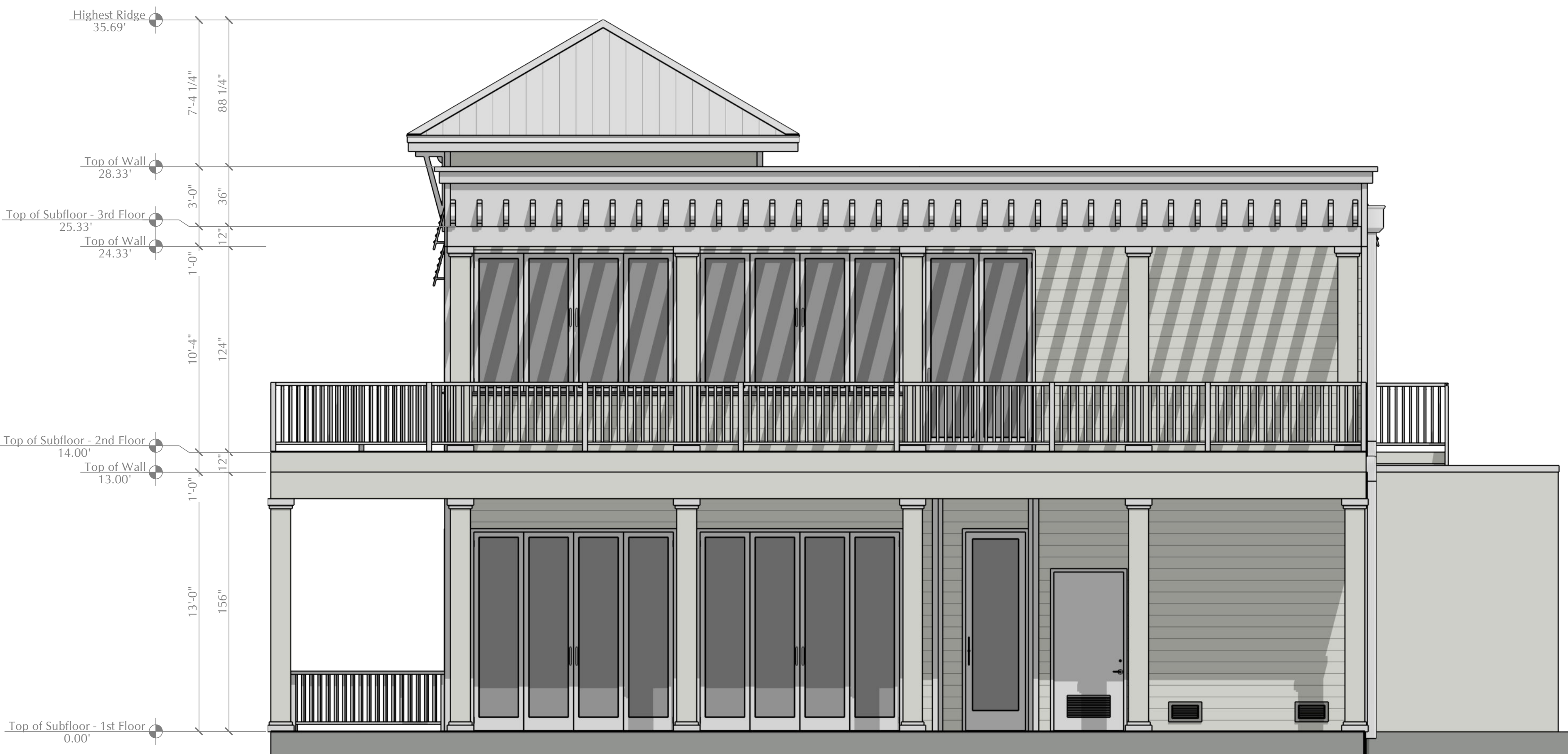
E4 - RIGHT (SOUTH) ELEVATION Scale: 1/4" = 1'-0"
