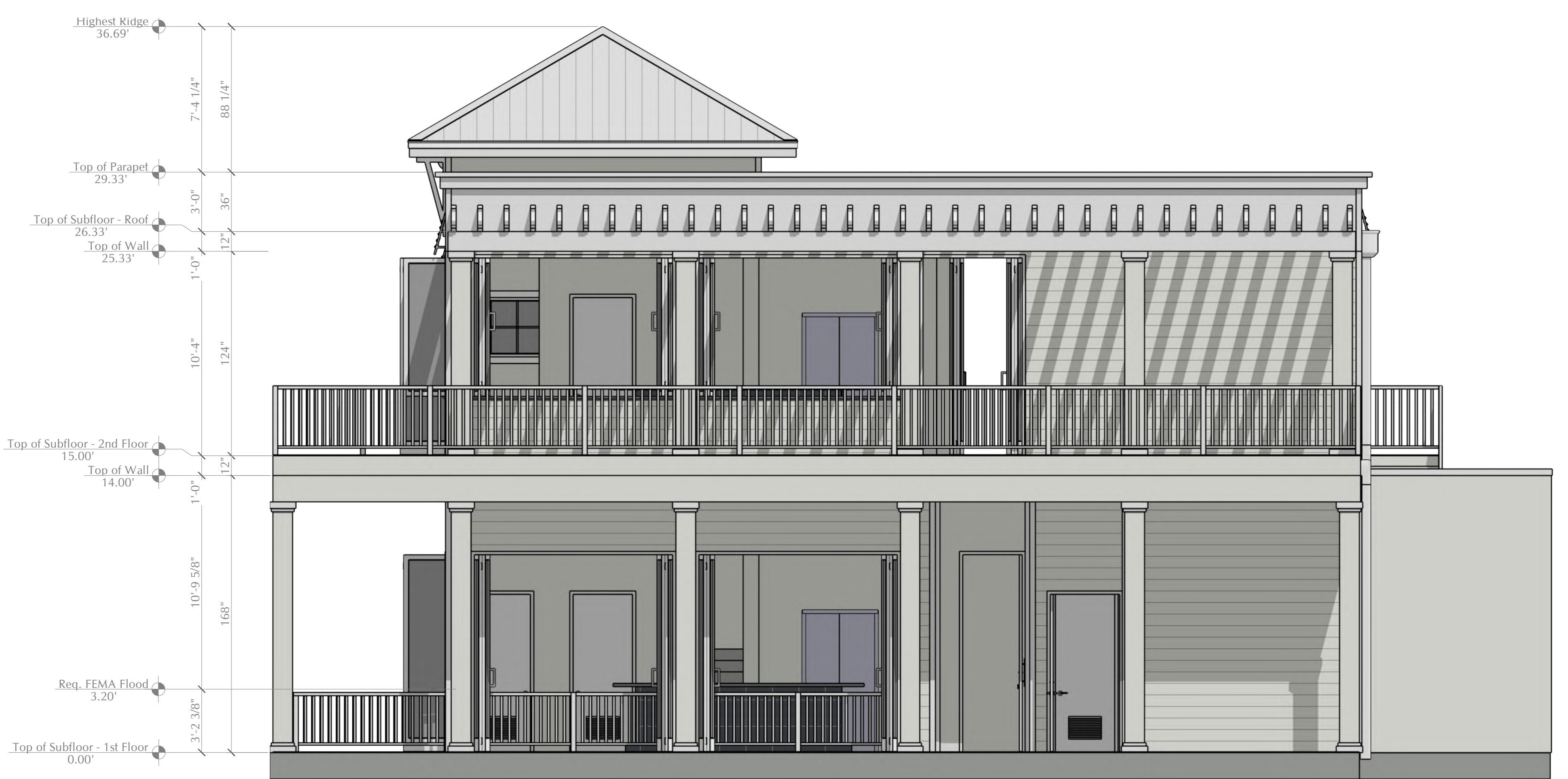
E4 - RIGHT (SOUTH) ELEVATION Scale: 1/4" = 1'-0"
